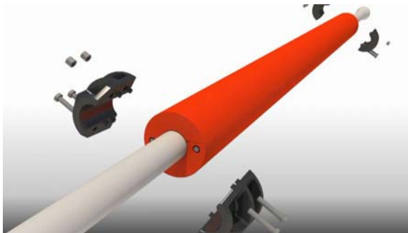
Illustration 1. - A joint of landing string with buoyancy modules installed
