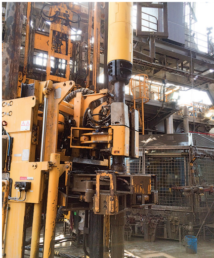
Fig. 4. A buoyancy-enhanced landing string being run in hole.
