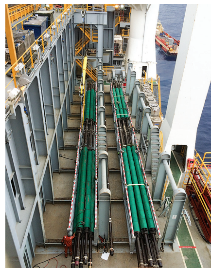
Fig. 2. The baskets holding the color-coded LSS doubles, to designate pressure ratings, were arranged sequentially on the pipe deck, in the order that they were to be run into the well.
