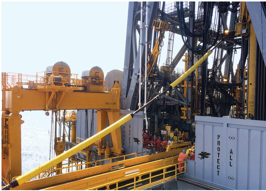
Fig. 3. An LSS double being picked up for running in the hole.
